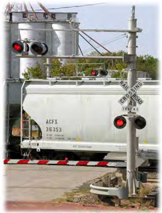
Figure 10.8 Gate / Multiple Railroad Tracks
